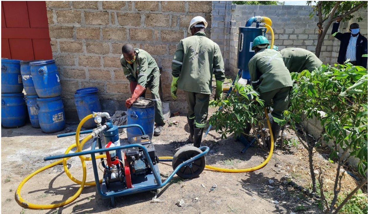
FIGURE 8: THE PITVAQ, A PORTABLE VACUUM PUMPING MACHINE DEVELOPED IN SOUTH AFRICA FOR EMPTYING PITS AND SEPTIC TANKS IN HARD TO REACH PLACES. THE PITVAQ IS USED IN CONJUNCTION WITH 50 TO 60 LITRE SEALABLE SLUDGE DRUMS, WHICH CAN BE RELATIVELY EASILY AND HYGIENICALLY CARRIED AND TRANSPORTED.
