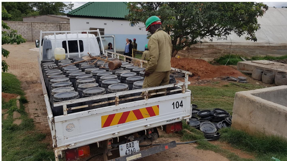
FIGURE 11: PIT SLUDGE IN LUSAKA IS TRANSPORTED IN SEALED 50 LITRE DRUMS.
