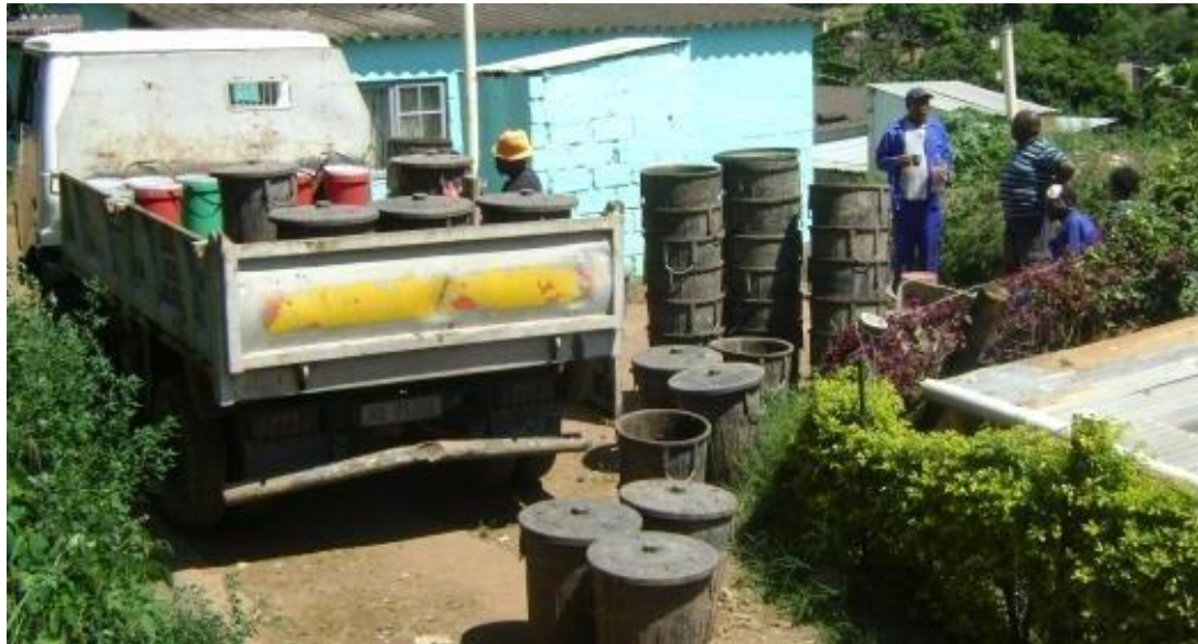
FIGURE 10: TRANSPORT OF PIT SLUDGE IN DURBAN PIT EMPTYING PROGRAMME (NOTE: IT IS BETTER PRACTICE IS TO USE 50 LITRE DRUMS WITH SEALABLE COVERS AS SHOWN IN THE FIGURE 11 BELOW)
